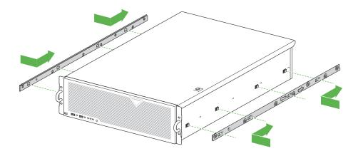
2. Align the four cutouts over the four hooks on the outside of the Violin 6000 Series Memory Array chassis and then slide the inner rail section toward the rear of the chassis until it is securely in place.
