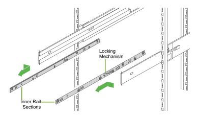
2. Press the spring-loaded lock mechanisms on the outside of both inner rail sections and then pull out and remove the inner slide rail sections from the left and right slide rails.
